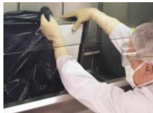
Filter cartridges guarantee safe and easy filter replacement
