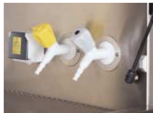
Filter cartridges guarantee safe and easy filter replacement
